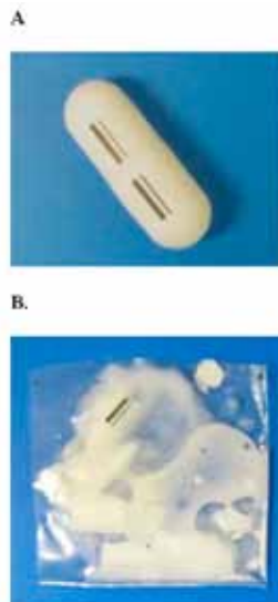
Figure 1. An intact ORADUR capsule (1A) and freeze fracture resistance of capsule following a crushing action (1B).
